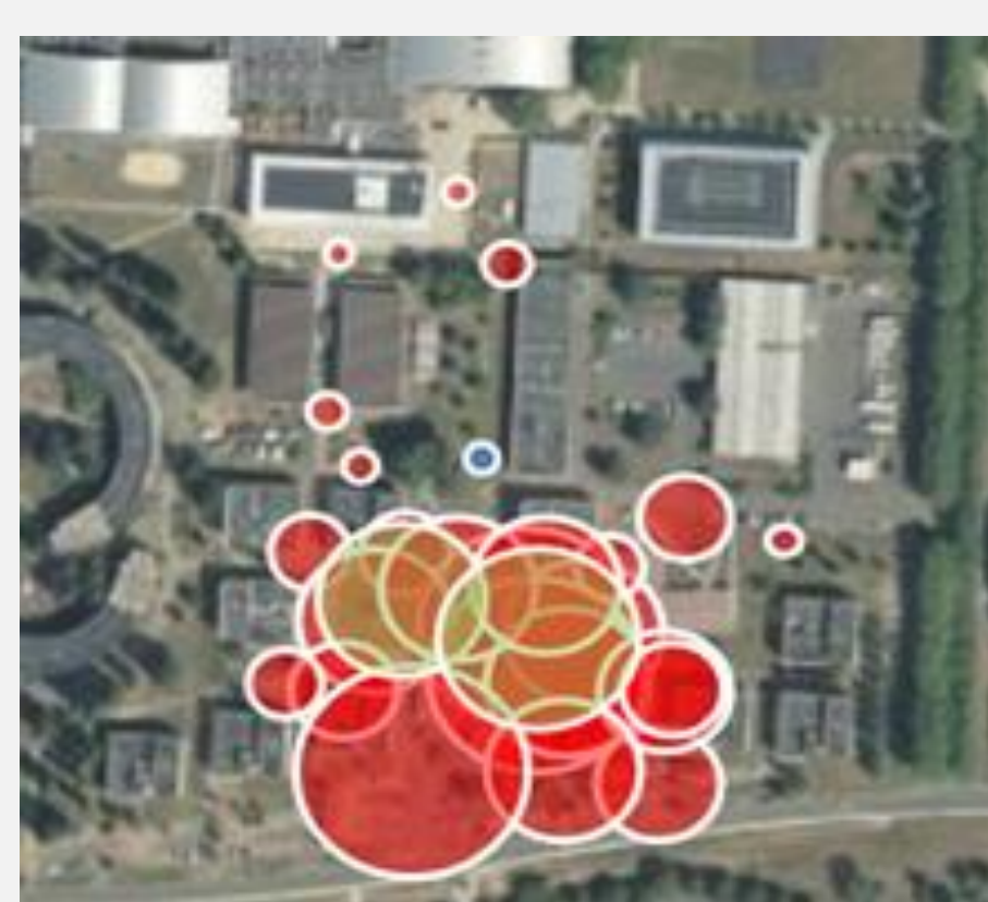
He plume dispersion based on ATC distribution. Wind speed 1.4 m.s -1 at 30 m ● Emission point ● ATC at sampling point ● ATC at real time The bubbles size is proportional to the ATC
