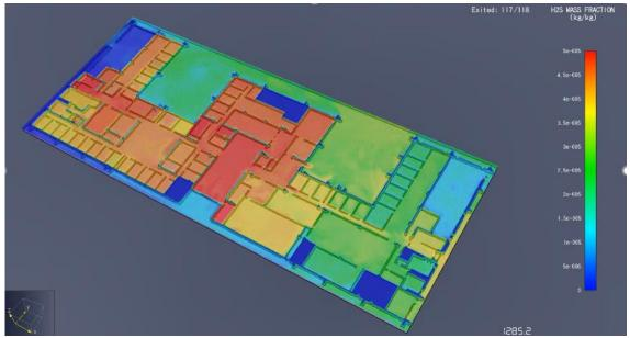
Figure 1: LES modelling of indoor dispersion of H<sub>2</sub>S in the administration building.
