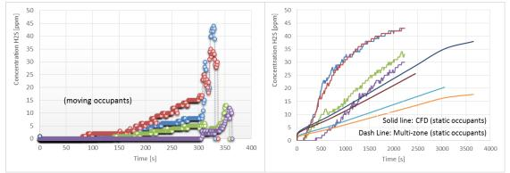
Figure 3. Toxic load estimation of the moving evacuees after a delay of 300 s: a) CFD results for moving occupants and b) CFD vs multi-zone (CONTAM) results for static occupants.
