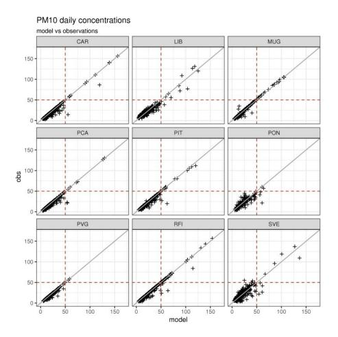
Figure 2. Validation of the hybrid modelling suite against data measured by the stations of the monitoring network. Scatter plots of daily mean concentrations. Most of these observed data are used to feed the universal kriging, in the last step of the modelling procedure, but the station "Via Svevo" (SVE) was kept out; therefore, the SVE panel (bottom right) shows a validation against independent data.
