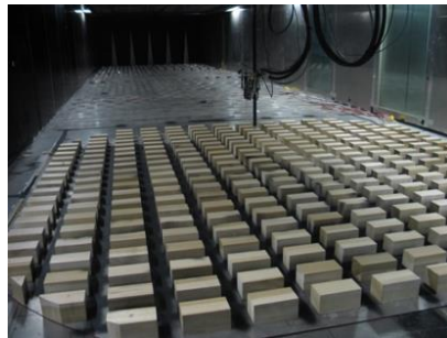
Figure 1. Looking upstream in the wind tunnel. The array is in the \theta = 0^\circ orientation
