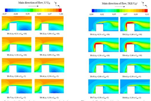
Figure 3. longitudinal velocity contour in vertical plane xz at y=(0.0).
