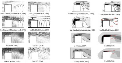
Figure 5. Vector field in plane of symmetry.
