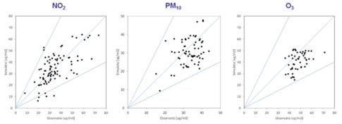
Figure 3. Annual average concentration values from the 4 km grid step simulation in the Corteolona study, compared to values measured in 2010 by ARPA Lombardia regional monitoring network
