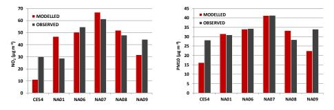
Figure 4. Annual average concentration values from the 1 km grid step simulation in the Acerra study, compared to values measured in 2013-2014 by ARPA Campania regional monitoring network
