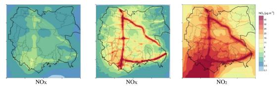
Figure 5. Overall annual average concentration values for nitrogen oxides on the "local" domain in the Acerra study. From left to right: NO<sub>X</sub> from local sources modelled with FARM at 1 km resolution; NO<sub>X</sub> from local sources modelled with SPRAY at 250 m resolution; NO<sub>2</sub> from all sources as sum of the contributions of both models.
