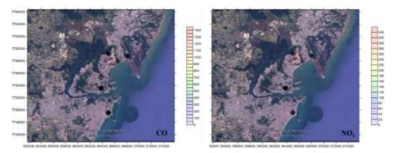
Figure 3 – Dispersion of CO and NO<sub>x</sub> emitted from vehicles. Concentration values are in µg/m<sup>3</sup>.
