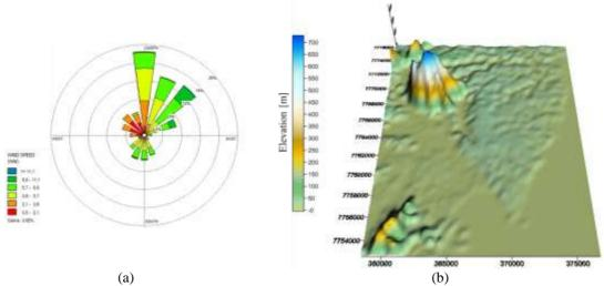
Figure 1 - (a) Wind rose: data represent an annual average; (b) Digital elevation model of the studied region
