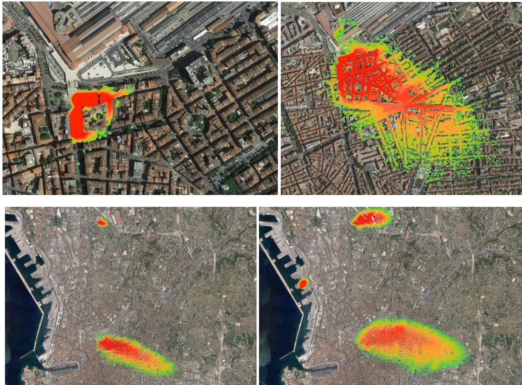
Figure 6: Concentration field near ground 3, 15, 38mn and 1h15mn after the first release time (from top left to bottom right).
