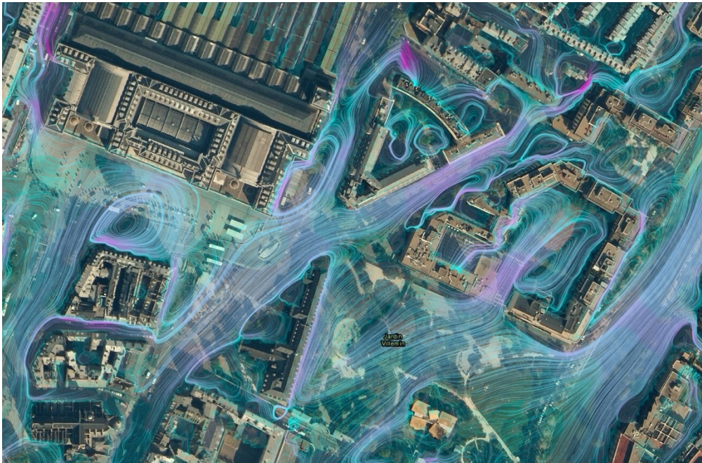
Figure 3: Streamline web display of wind field in streets of Paris at zoom level 17
