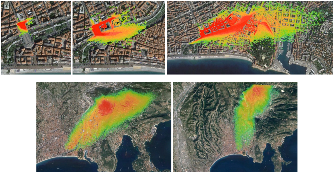
Figure 5: Concentration field near ground 2, 5, 15, 55mn and 1h30mn after the release time (from top left to bottom right).
