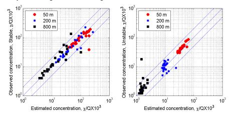
Figure 1. Comparison of numerical solution of diffusion equation with measurements from Prairie Grass
