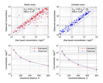
Figure 3. Comparison of maximum concentration measurements made during the Prairie Grass Experiment at 50m, 100m, 200m, 500m, and 800m from the release with model estimates based on Equations (14) and (15). Bottom panel shows the variation of the average of the maximums measured on each sampling arc.
