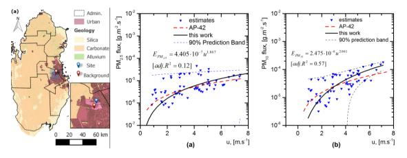
Figure 1. Details of the emissions field study (inset) and the developed (a)  $PM_{2.5}$  and (b)  $PM_{10}$  emission factors for the local surface soil type (i.e. calcisols) (Hassan *et al.*, 2016).
