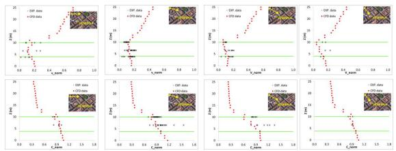
**Figure 3.** Experimental and modelled vertical profiles of normalized horizontal wind speed (top pannels) and BC concentrations (bottom pannels) for different inlet wind directions in the street with trees.
