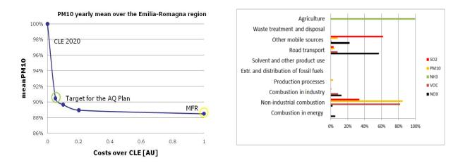
**Figure 2:** Pareto curve for the optimisation of yearly average concentration of PM10 (MFR is the maximum feasible reduction) and the corresponding emission reductions over CLE2020
