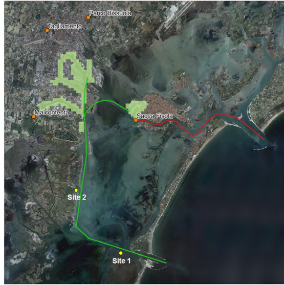
Figure 1. Itinerary of the ships > 40kTon in the Venice Lagoon. Red line: present S0 scenario (Giudecca canal); green line: future S1 scenario (Malamocco- new Tresse canal); red circles: locations of the measuring stations; yellow circles: additional analysis sites
