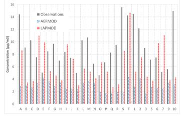
Figure 3. Period averaged concentrations for observations, AERMOD, and LAPMOD predictions.
