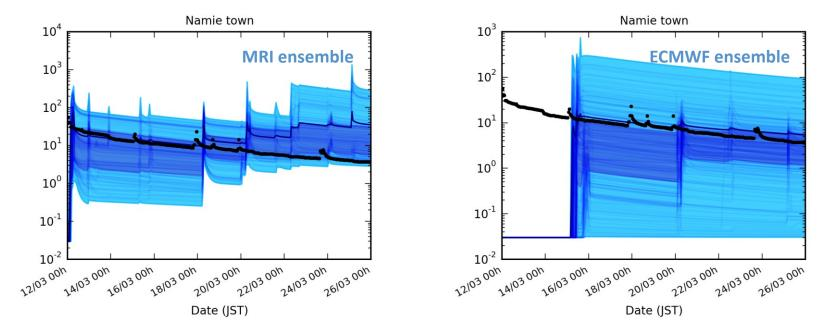
The spread of the simulations ensemble is quite large compared to the observation variation. The small variability of the meteorological data allows to create large variability in the dispersion results.
