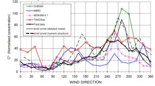
Figure 4 Normalised concentrations versus the wind direction calculated by 4 CFD codes and measured in the full-scale experimental site and in the wind tunnel.
