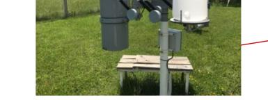
Automatic samplers for wet and dry deposition (WADOS - Kroneis GmBH)
