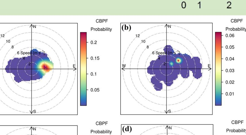
The NO<sub>x</sub> pollutant roses for the four simulation periods performed using SWIFT wind data for the source point at the plant stack elevation and the hourly NO<sub>x</sub> ground simulated concentrations in a 100 m x 700 m area over the Eastern slope of Mount Titano were used to obtain conditional bivariate probability functions (CBPF) (figure at left).
