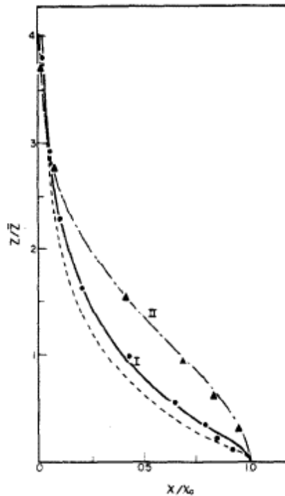
Fig. 3. Comparison between the shape of the measured and calculated concentration profile; I. Run 26: L^{-1} = -0.031 \text{ m}^{-1} ; ● measurement, — computation with K_x = 1.35 K_M , --- computation with K_x = K_M ; II. Run 59: L^{-1} = 0.095 \text{ m}^{-1} , ▲ measurement, - · - · computation with K_x = 1.35 K_M and K_z = K_M .
