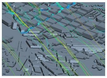
Perspective view of the wind lines in Pamplona when the wind blows North direction.
