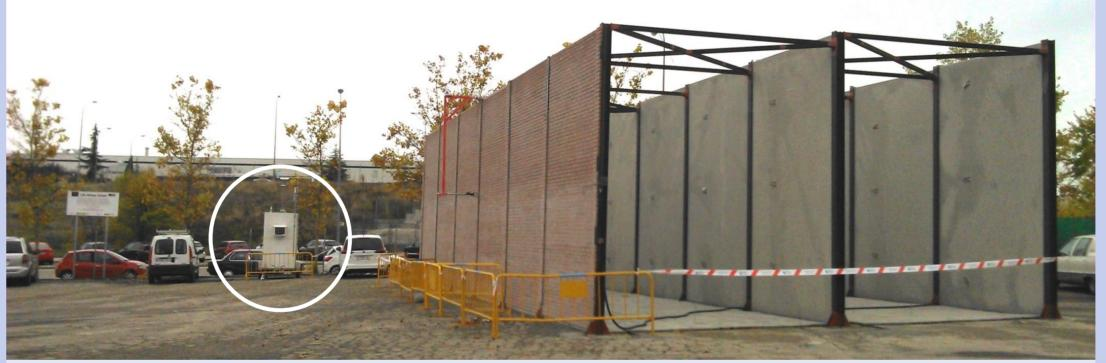
A mobile monitoring station (marked in the image) was installed near the street canyon for the continuous measurement of NO, NO<sub>2</sub> and O<sub>3</sub> concentrations and meteorological parameters in both scenarios measurement in order to document the evolution of the physical chemical characteristics of the air mass existing in the zone and obtain fundamental information for a correct interpretation of the results.
