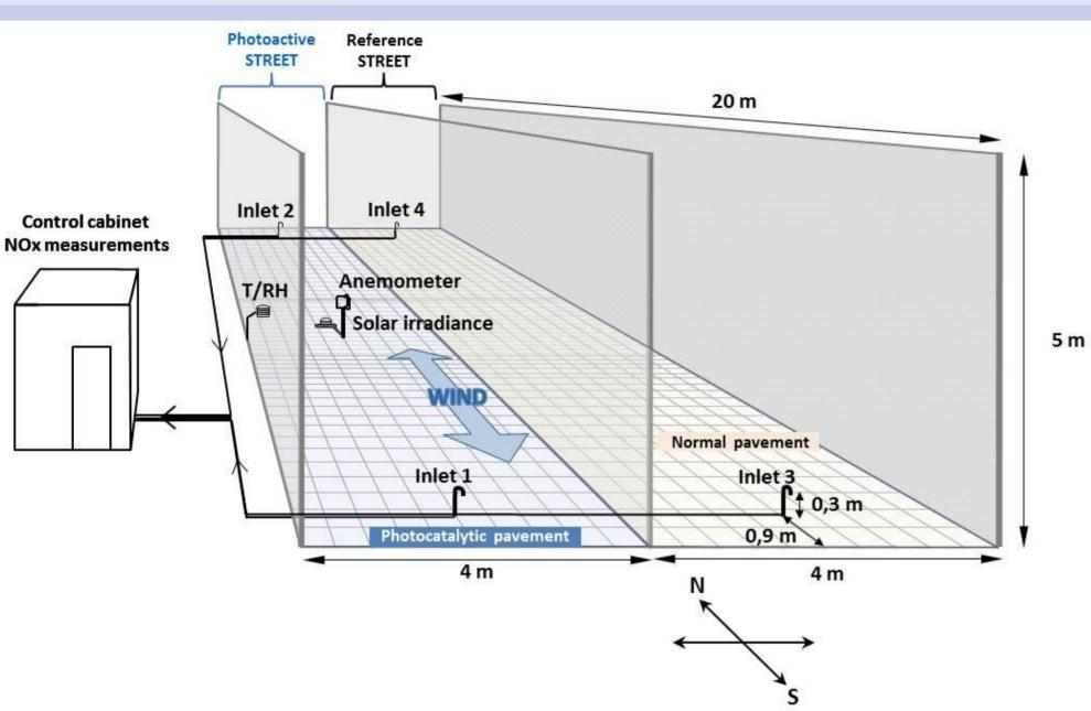
Scheme of the experimental set up Photoactive street: Sampling points 1-2 and meteorology sensors Reference street: Sampling points 3-4 Control cabinet: Continuous measurement of NO, NO<sub>2</sub> (Thermo Scientific 42i) Experimental campaign: April, 6<sup>th</sup> 2016 till June, 30<sup>th</sup> 2016
