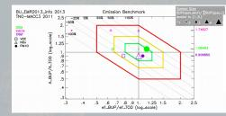
**diamond diagram**: it is designed to identify discrepancies between inventories; it allows to assess whether the differences can be mostly related to different emission factors or in the choice of activity data
