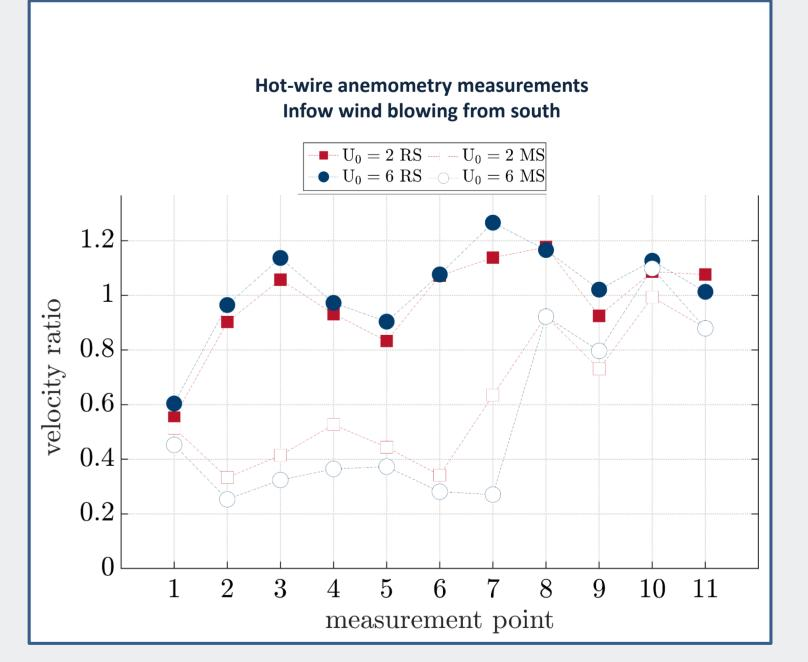
The results show a reduction of wind speed between 4 and 6 m.s<sup>-1</sup> within the auditorium, with the mitigation measures. There is also an attenuation in recirculation near the wall, upstream from the auditorium, leading to an effective reduction of the wind speed.
