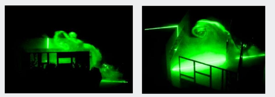
The turbulent flow is accelerated upstream the auditorium, as a result of the street canyon configuration of the surrounding avenue, followed by a deceleration of the flow induced by the vegetation.
