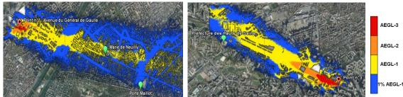
Figure 1. Distribution of a toxic chemical released in "La Defense" district (results given for two release locations). The danger zones have warm colours. They were determined using the AEGLs of the US-EPA.
