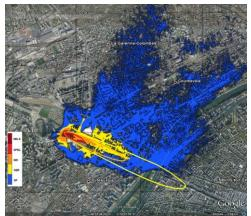
Figure 3. Comparison of the danger zones predicted by PMSS and ALOHA.
