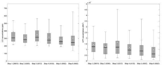
**Figure 4.** Distributions of observed CO (left) and UFP (right) concentrations from all mobile measurements in Woodside. Each distribution is based on n observations (shown below). The middle line represents the median, the box the 25th and 75th percentiles, and the whiskers the 5th and 95th percentiles. The point represents the mean value of the distribution.
