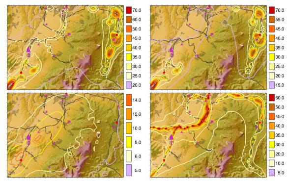
**Figure 1.**Annual concentrations of PM<sub>10</sub> (upper left), PM<sub>2.5</sub> (upper right), SO<sub>2</sub> (lower left) and NO<sub>2</sub> (lower right) modeled by CALPUFF. Red pentagons are monitoring stations, pink triangles are industrial point sources and black lines are major roads.
