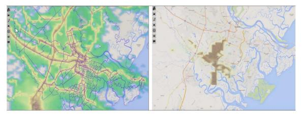
Figure 1. Example screen shot from C-LINE showing modelled near-road pollutant gradients (left) as well as the change in PM<sub>2.5</sub> concentrations resulting from emissions changes (right).
