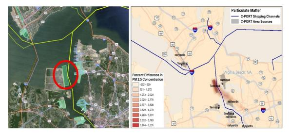
Figure 2. Example screen shot from C-PORT showing planned construction of Craney Island to increase container volumes at Panama Canal (left) as well as the change in PM2.5 concentrations (%) resulting from the proposed expansion (right)
