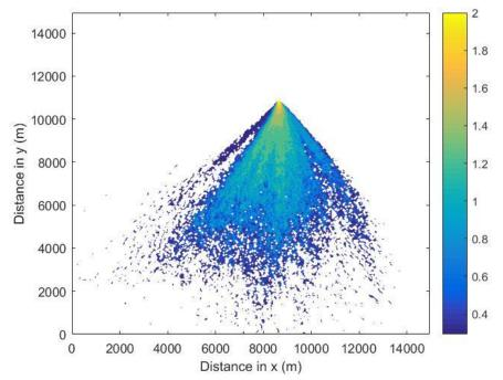
Figure 3. The probability in space of the plume-passage for the LHS-perturbed ensemble plotted in a logarithmic scale. Hundred percent corresponds to 2 and ten percent to 1.
