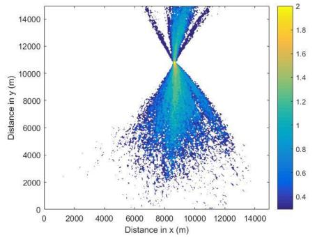
Figure 4. The probability in space of the plume-passage for the shifted LHS-perturbed ensemble plotted in a logarithmic scale. Hundred percent corresponds to 2 and ten percent to 1.
