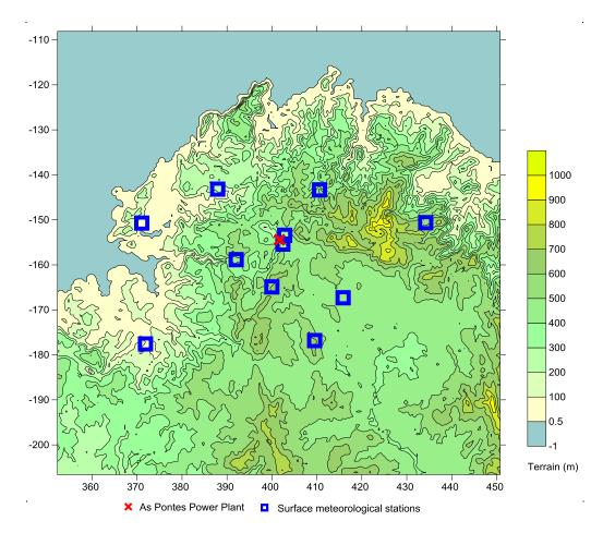
Figure 1. Location (UTM coordinates) and digital elevation model (asl-m) of the CALMET simulation domain inside the D3 domain (Northwestern Galicia), with the location of meteorological surface sites for model assessment. Terrain values [-1,0.5] correspond to sea level.
