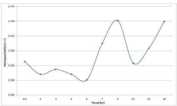
Figure 3. Wind speed RMSE variation from CALMET simulations using with different TERRAD values
