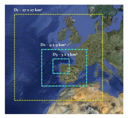
Figure 2. WRF nested domains, including D3 domain that provides the meteorological input to CALMET simulations.
