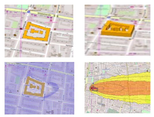
Figure 1. a, b, c, d. Scenario building block. Figures show 2 d- and 3 d- sight (top left, top right), windfield (wind direction 270°) and inhalation dose for an arbitrary radionuclide and activity (bottom left, bottom right).
