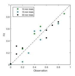
Figure 2. Predicted vs. observed fractional casualties for all the subset of 20 steady-exposure trials with T = 10, 15, and 30 minutes. The predictions used toxic load model coefficients that were fitted using the same subset of data.
