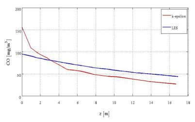
Figure 7. CO concentration along the vertical line, in correspondence of the measuring point.
