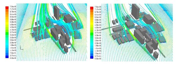
Figure 4. Comparison of the streamlines obtained over the built area with the k-epsilon model (left) and LES (right).
