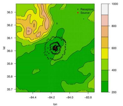
Figure 1. Topography, receptors positions on 4 arcs and source position (centre of the figure).
