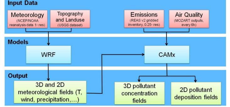
The WRF-CAMx system was built over a coarse domain covering southeast coast of China (9 km<sup>2</sup> horizontal resolution) and a nested domain with 3 × 3 km<sup>2</sup> resolution (over the PRD region).
