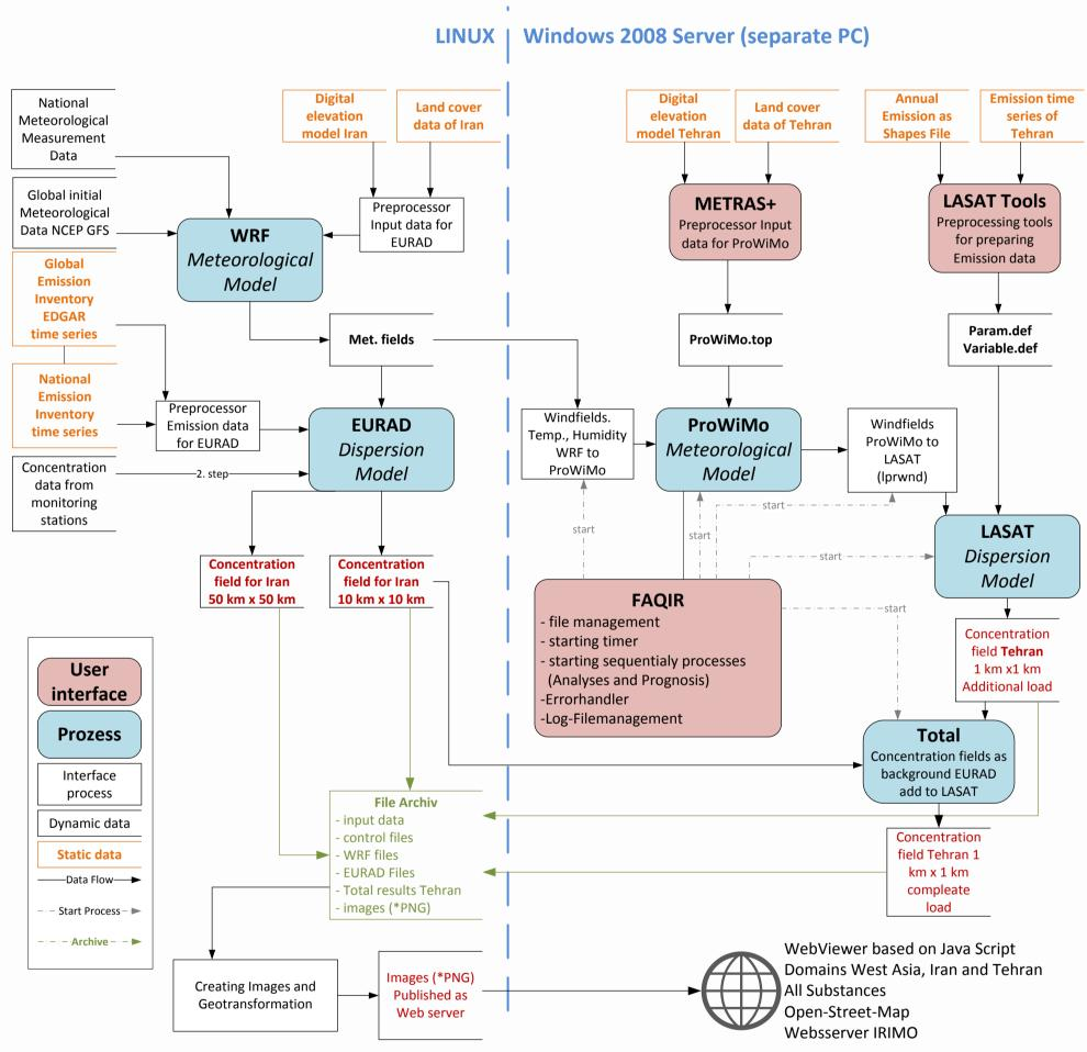
For the urban regions of Tehran, the PROWIMO simulation domain has a horizontal extent of 90 x 90 km<sup>2</sup>. The horizontal grid size within an inner domain of 50 x 50 km<sup>2</sup> (Domain D02.1) is 1 km. Outside of that inner domain the horizontal grid size increases with a factor of 1.2. A vertical grid size of 20 m has been chosen from surface up to a height of 120m, above the vertical grid size increases with a factor of 1.2.
