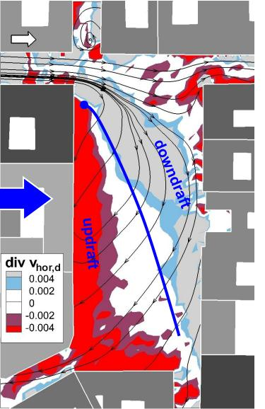
VERTICAL COMPONENT CALCULATED FROM WIND TUNNEL (LDV) RESULTS
