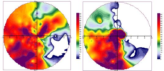
*Fig. 5: Polar plots of mean NO<sub>X</sub> concentration at monitor LHR2. (Left) Monitored concentration (Right) ADMS-Airport concentration. Axes show wind speed from 0-10m/s.*
