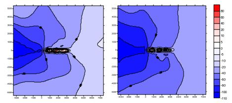
*Fig. 3:* A340. Percentage difference in annual average ground level concentration between an A340 modelled as twin-engined and 4-engined (left) 1-engined and 4-engined (right). Only wind directions from 180° to 360° have been modelled.
