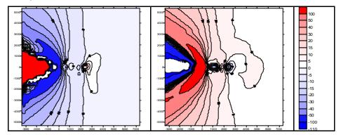
Fig. 4: A320 Percentage difference in annual average ground level concentration between an A320 with jet exhaust increased by 50% (left) decreased by 50% (right) compared with concentration due to a jet with the unmodified velocity.
