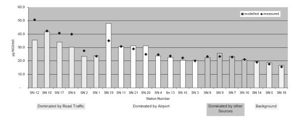
Fig. 5; Local air quality studies. Modelled versus measured  $NO_2$  concentration (annual mean) at different monitor stations around Zürich Airport (Fleuti, E. and P. Hofmann, 2005).
