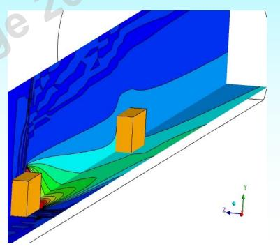
Entrapment to the wall side wake region with higher than expected concentrations in locations in the wake region compared to the single bus
