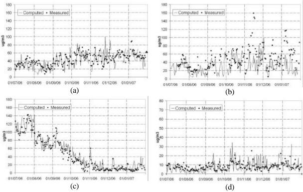
Fig. 5; Comparison between measured and computed daily average ground concentration levels. (a) NO<sub>2</sub> concentrations, Novara – Via Leonardi monitoring site (b) PM<sub>10</sub> concentrations, Novara – Via Verdi (c) O<sub>3</sub> concentrations, Novara – Via Verdi (d) SO<sub>2</sub> concentrations, Novara – Via Bovio.
