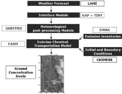
Fig. 2; Interconnection between modules that constitute the ARIANOVA system.
