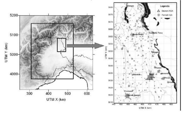
Fig. 1; Outermost and innermost computational domains employed for the forecast modelling system.
