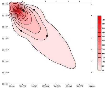
Fig. 5; Contamination thickness distribution downwind from chlorine leaking spot
