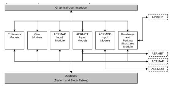
Fig. 1; EDMS system architecture and components.
