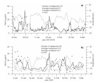
Figure 3. Comparison of measured (+) and modelled (grey solid line) daily mean concentrations of PM10 ( $\mu$ g/m<sup>3</sup>) at Lycksele/Sweden for two different time periods. Grey broken line is background concentrations and thin grey solid line is daily mean temperature. (a) Time period 20011214-20020310, (b) Time period 20060101-20060310.
