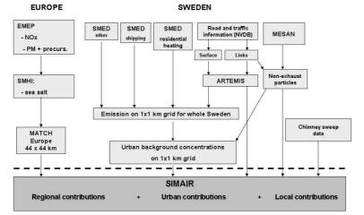
Figure 1. Databases and models used by the SIMAIR system. The dashed line illustrates the difference between stored data and precalculated concentrations from models of larger scale which is done on a Linux server (above the dashed line) and local models and user interface accessed from an ordinary Internet browser (below the dashed line).
