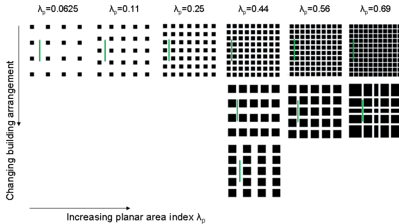
Figure 1. Diagram showing increasing planar area index \lambda_p and changing building arrangements of the arrays investigated. The wind blows from left. The line source is positioned along the first upstream buildings line.
