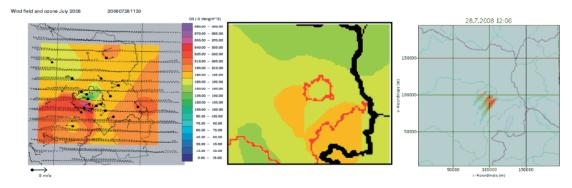
Figure 5. Left: Observed wind and ozone concentrations on 28th July at 11:30. Middle: Ozone forecast (ALADIN-CAMx) for the 28th July 12:00 2006. Right: Calculated dispersion of the plumes of the dominant industrial NOx sources in Vienna.
