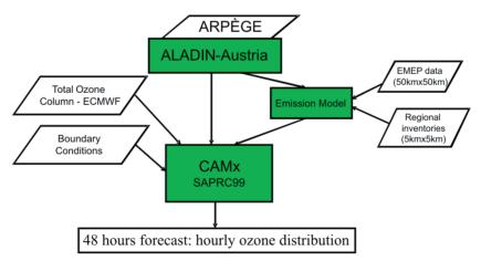
Figure 1. ALADIN-CAMx – air quality modelling system.
