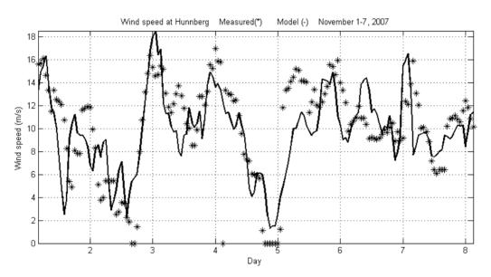
Figure 3. Measured (sodar (\*)) and simulated (-) wind speed at site Hunneberg at 175 m.
