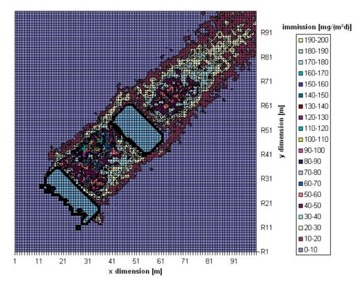
Figure 3. Immission of PM10 in simulation area.
