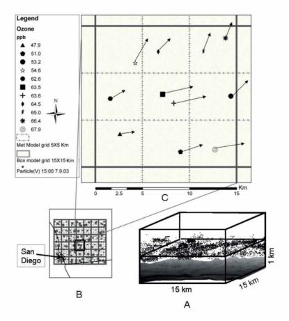
Figure 1. Illustration of the grid structure for the hybrid modeling system (atmospheric, Lagrangian, and box chemistry models) with an example of one chemical component – ozone.
