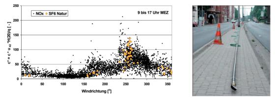
Figure 3. Normalized half-hourly mean concentration as a function of wind direction (left hand side). Black data points represent measurements of traffic generated  $NO_x$  immissions, yellow data points represent corresponding  $SF_6$  immissions originating from the artificial line source shown in the right hand side figure.
