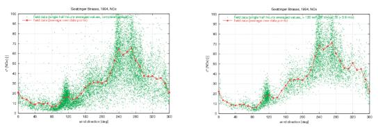
Figure 2. Normalized half-hourly mean concentration values as a function of wind direction measured over a period of one year at the street monitoring station 'Goettinger Strasse' in Hanover/Germany. Unfiltered (left hand side) and filtered (right hand side) data, see text.
