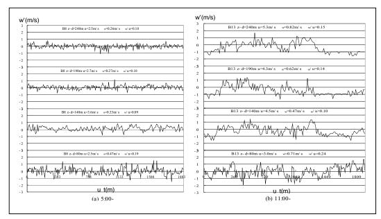
Figure 3. w'at (a) 5:00 - 5:15 and (b) 11:00 - 11:10 on 19 July (2007) measured using Doppler sodar at the centre of Himeji city.
