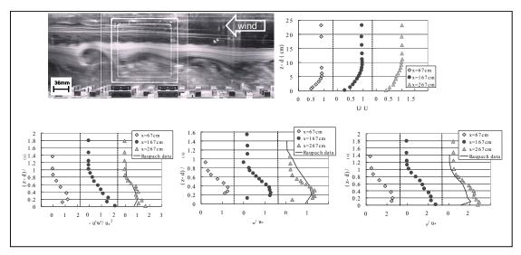
Figure 6. A visualization of the urban boundary layer and  $U/U_{\infty}$ ,  $-u'w'/u_*^2$ ,  $\sigma_w/u_*$ ,  $\sigma_w/u_*$  in the wind tunnel.
